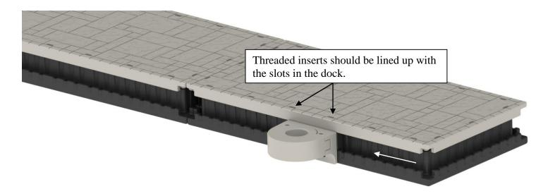
4. Install pylon to complete the installation.
